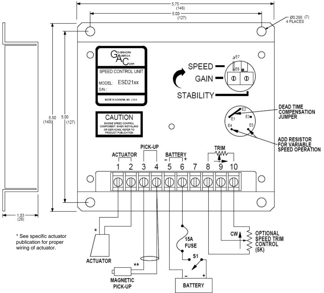
\*\* If wire leads are longer than 3 meters (10ft) a shielded cable should be used. Ground shield at one end only.
